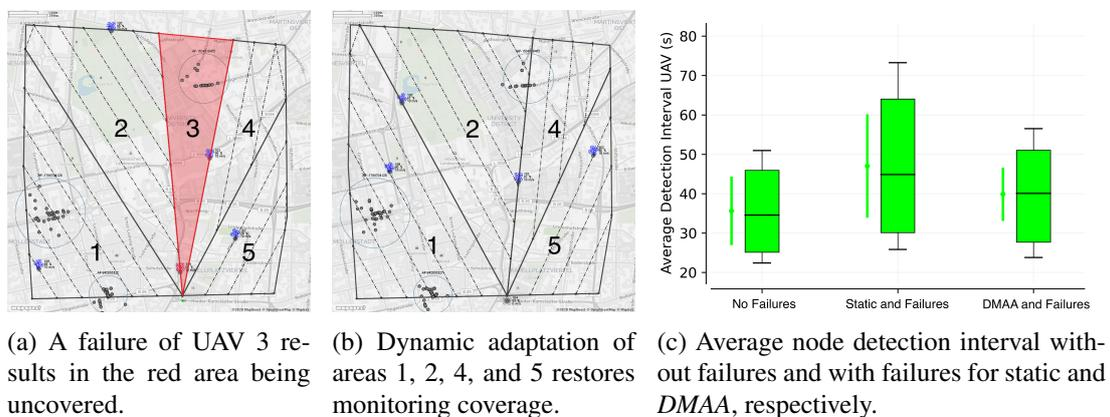
Figure 2: *Dynamic Monitoring Area Allocation* improves resilience against UAV failures.
