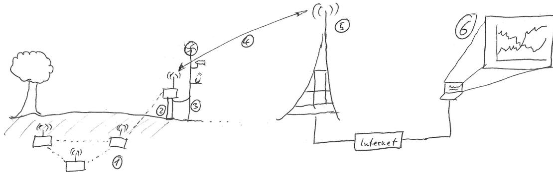
Figure 1: The Infrastructure of the demo setup: The measured data is transmitted from the MoleNet nodes to the end-user device.
