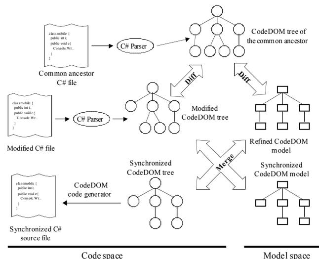
Fig. 6. Synchronization in the Windows Mobile platform
