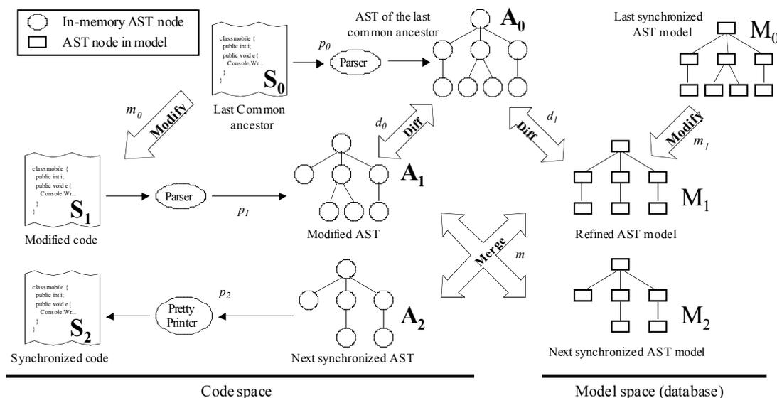
Fig. 3. Block diagram of the model-code synchronization
