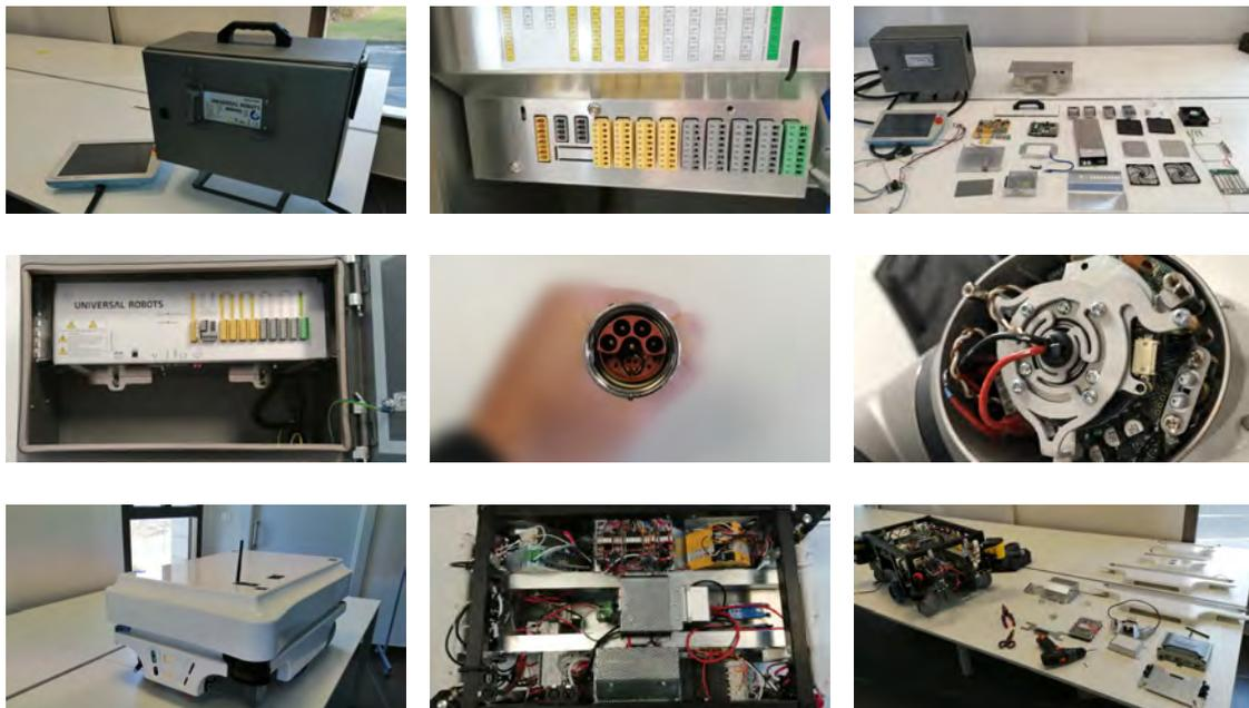
Figure 1: Teardown of three industrial collaborative robots: UR3 CB series (first three), UR3e-Series (fourth to sixth) and MiR100 (last three).
