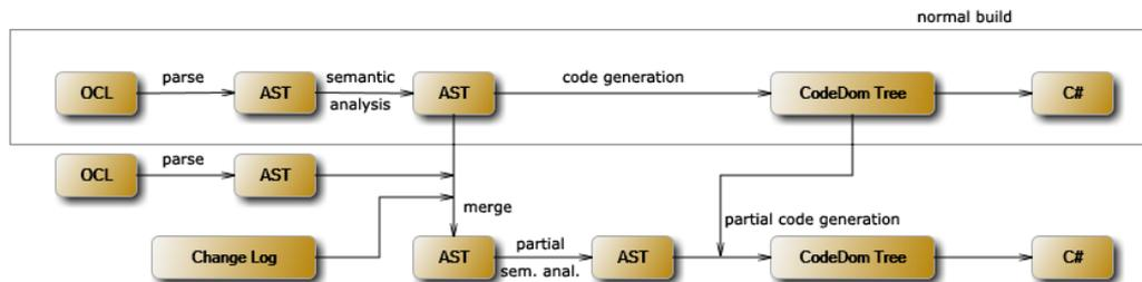
Figure 5: Data flow of the incremental compiler
