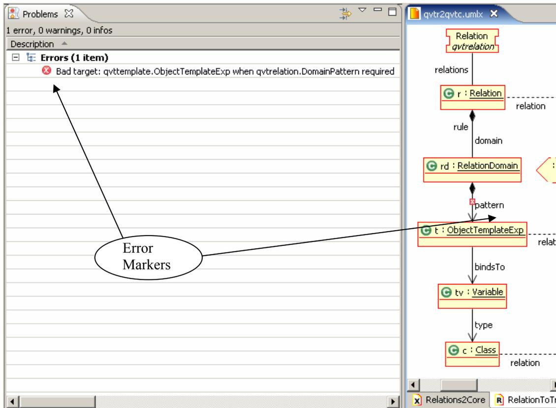
Figure 6 UMLX Views with errors
