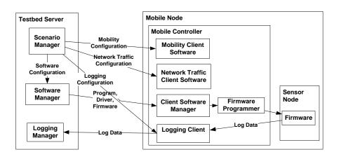
Figure 2: Interaction of Functional Blocks (Software)
