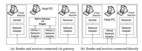
Figure 8: Test setup for evaluation
