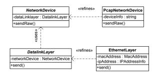
Figure 3: UML diagram showing the relation between DatalinkLayer, NetworkDevice and their refinements
