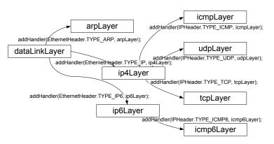
Figure 2: Network layers independently linked in EZnet
