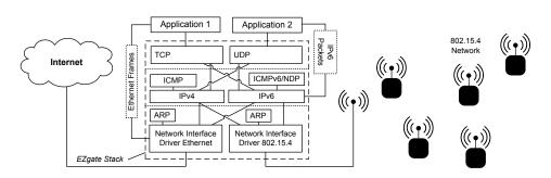
Figure 5: EZgate architecture example showing two network interfaces and two cross layer applications on top
