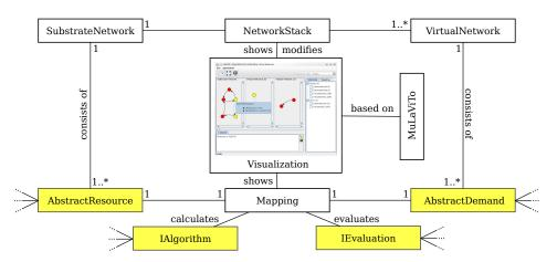
Figure 4: The framework ALEVIN and its modularity in parameters, algorithms, and evaluations.
