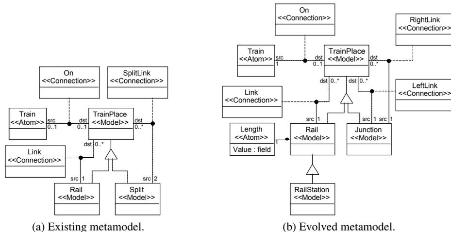
Figure 3: (a) The existing metamodel, and (b) the evolved metamodel, both modelled in GME. Class stereotypes indicate the type of model that will be instantiated in the language.
