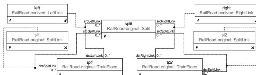
Figure 8: The customized migration transformation  $\mu'_{3,4,5}$  introducing the notion of direction. In this transform, items with a check are created, and items with an X are removed from the models.
