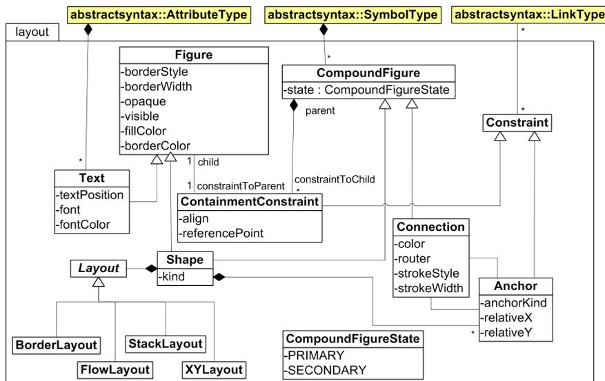
Figure 3: VL Specification: Concrete Syntax
