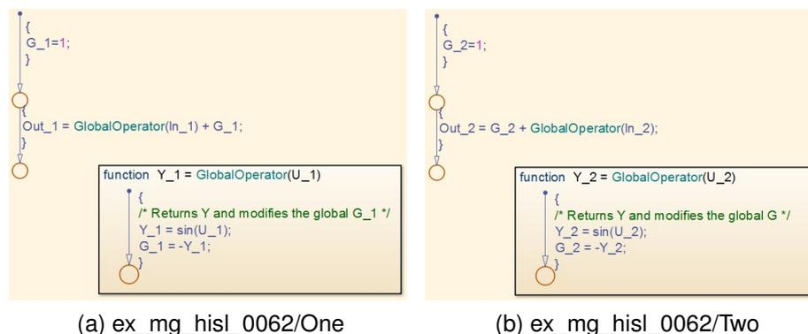
Figure 7: A Type 2 (renamed model clone), both (a) and (b) in the ex\_mg\_hisl\_0062 model. Simone similarity 81%.
